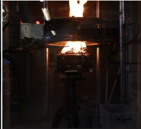
Figure 7 Visual observation of flaming combustion in cone calorimeter test
