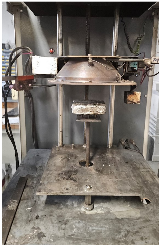
Figure 4 Testing area of a Cone Calorimeter
